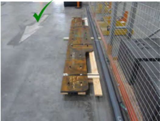
This steel section is well packaged and restrained.
