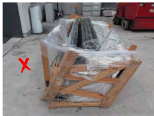
This crate is not strong enough for the contents and the contents are not blocked causing extra stress on the crate.
