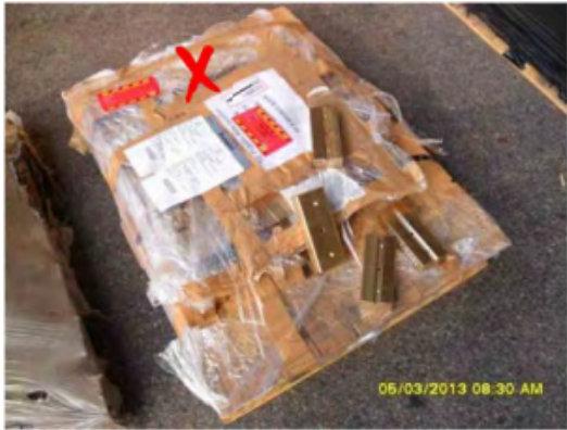
Shrink wrap was the only restraint applied to this load which proved inadequate prior to it being sent to site.
