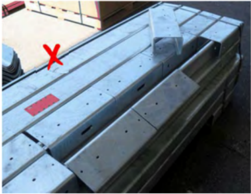
This load has not been restrained to prevent portions of it moving during handling.
