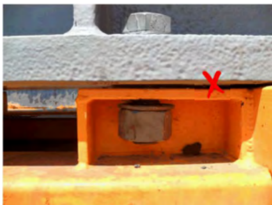
All mounting bolts must be tightened prior to despatch.
